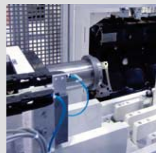
Force fit sealing parts and leak-test
